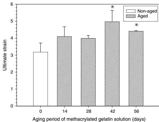
Fig. 5 Aging effects on the ultimate strain of freeze-dried films immersed in a 50% fetal bovine serum and 0.1% sodium azide solution maintained at 37°C for 4 days. Films were prepared with either a fresh (non-aged) or an aged 7.5 wt% methacrylated gelatin solution, the latter solution being stored for up to 56 days at room temperature. Data represent means \pm standard deviation ( n = 3 ). * Different from non-aged films ( P < 0.05 )
